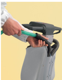
Periodical cleaning of squeegee hose to guarantee an efficient suction
