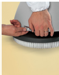
Before removing the solution tank don't forget to disconnect the water tube
