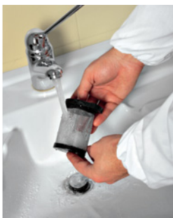
Thorough cleaning of the suction filter is easy and practical
