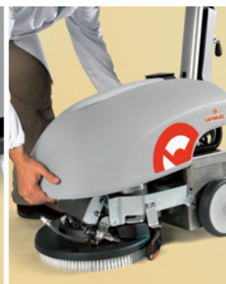
Before removing the solution tank don't forget to disconnect the water tube
